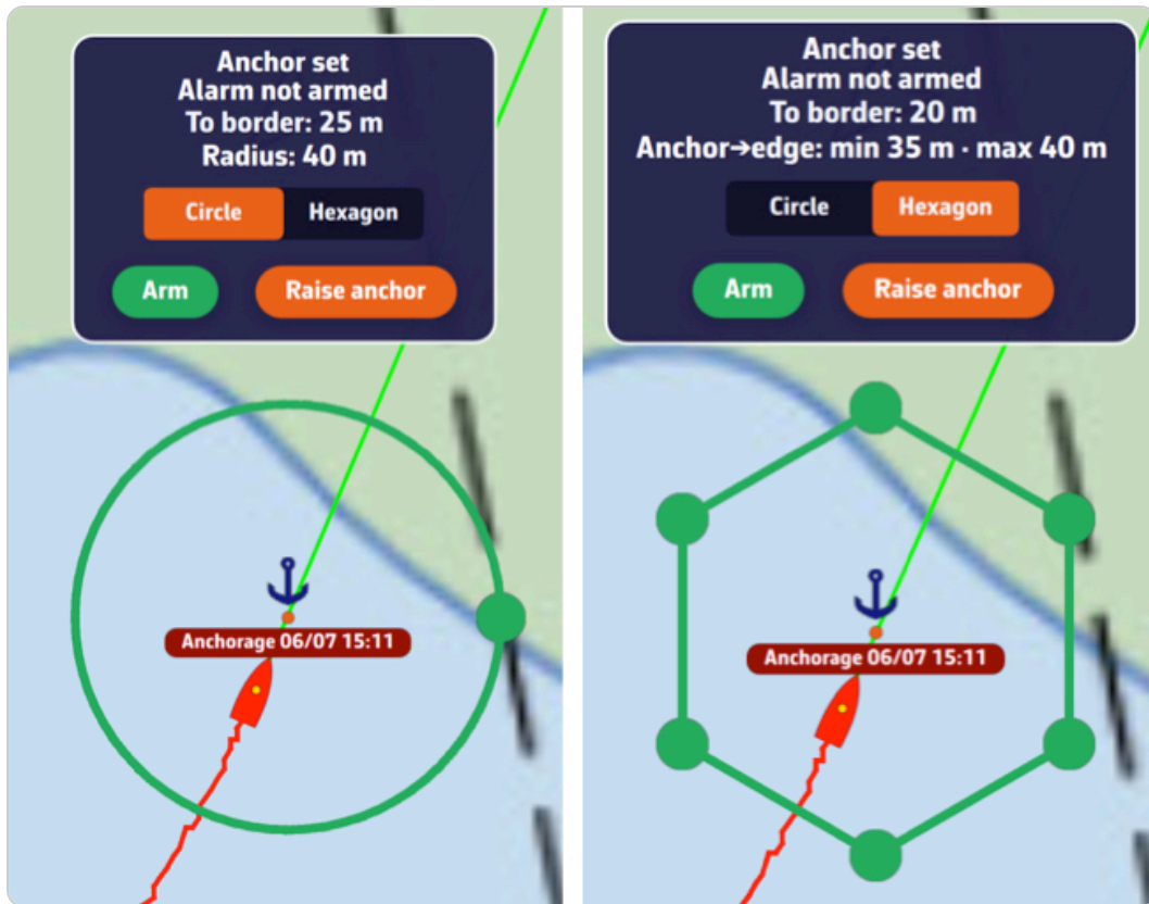
The anchor banner and the swinging zone, as a circle on the left and a hexagon on the right
