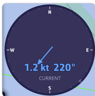
The Current rose: 1.2 kt at 220^\circ , the arrow shows where the current is setting
