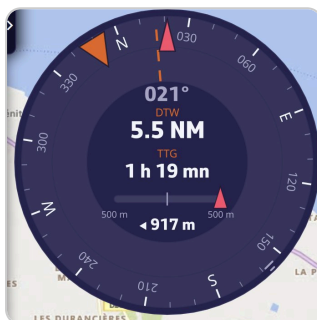
The Steering compass toward a POI: bearing to the waypoint, distance, time remaining and cross-track error bar
