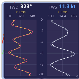
The Wind plot: true wind direction (TWD) and speed (TWS) side by side, with their dotted trend
