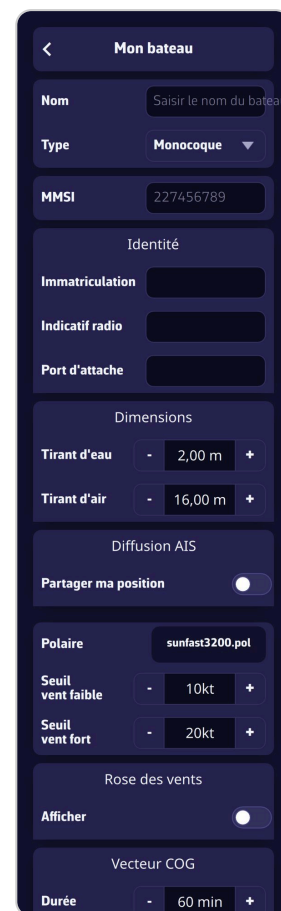
Settings > My Boat: name, type, MMSI, identity, dimensions, AIS broadcast, polar and wind thresholds
