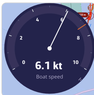
The Needle gauge on boat speed, with the polar's target speed marker
