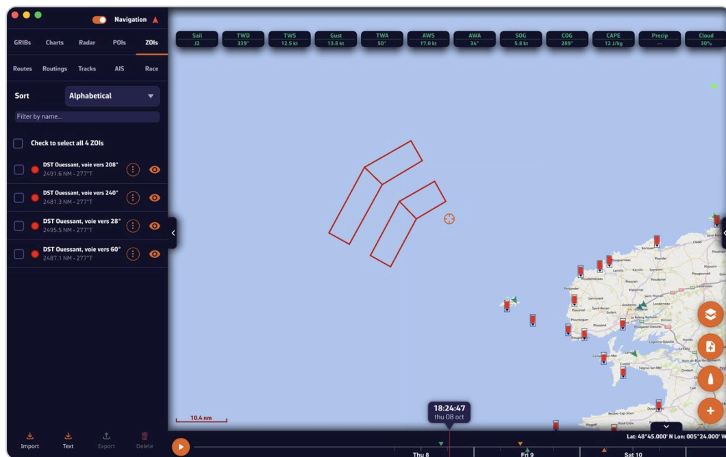
"ZOIs" tab of the left drawer and the lanes of the Ushant traffic separation scheme drawn in red on the chart
