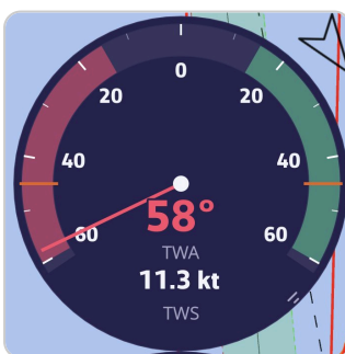
The Close-hauled wind: the wind angle needle on the expanded fan, with the wind angle and speed at the bottom
