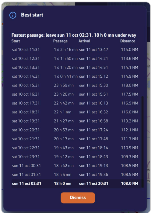
The "Best start" window at the end of the search: the fastest passage at the top, then the table of starts tried with the fastest in bold
