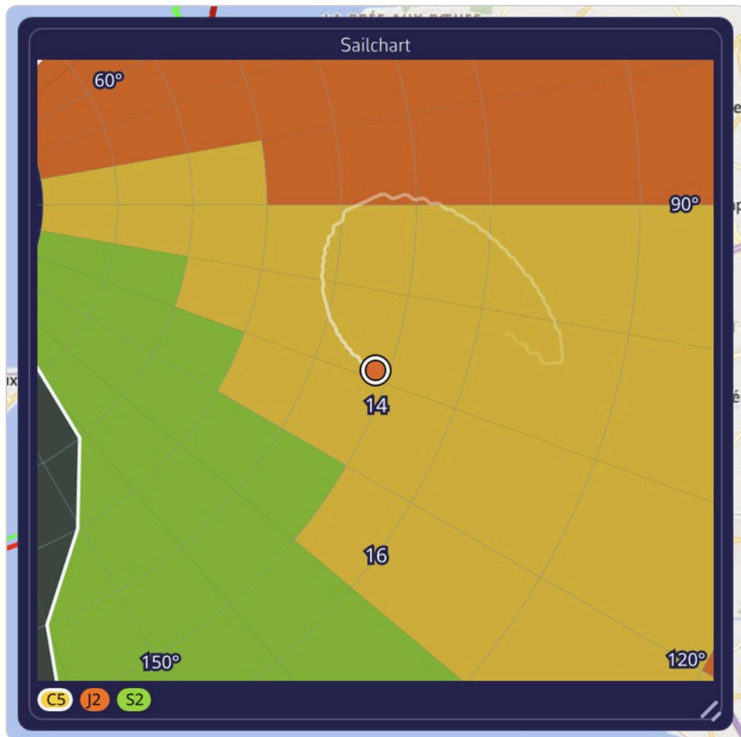
Sailchart instrument on the chart: the boat's orange dot and its track of the last ten minutes on the sail chart, sail legend at the bottom with the sail in use circled
