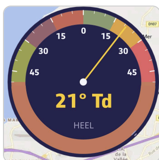
The Clinometer: heel on the \pm 50^\circ arc and its side, here on starboard tack
